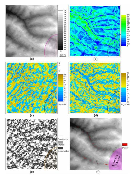
Fig. 1. Exploration of alluvial placers: (a) elevation, (b) slope factor, (c) horizontal curvature, (d) vertical curvature, (e) relative accumulation, transit, and dissipation zones, and (f) the most prospective areas. The primary deposit is hatched.
